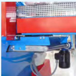
16 Belt for the recycling soil for tray filler.
