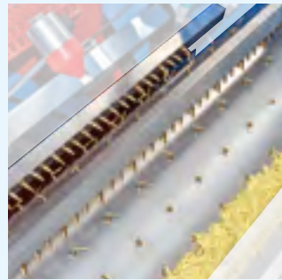
12 Seeding drum with raised nozzles for difficult seeds, for example tagetes, zinnia, etc.
